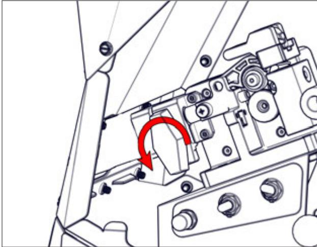
Loosen power pin connection knob
