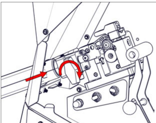
Tighten power pin connection knob
