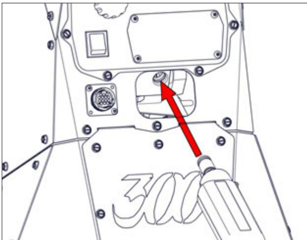
Install power pin connection of the gun. Verify the handle orientation is correct to not interfere with the sheet metal
