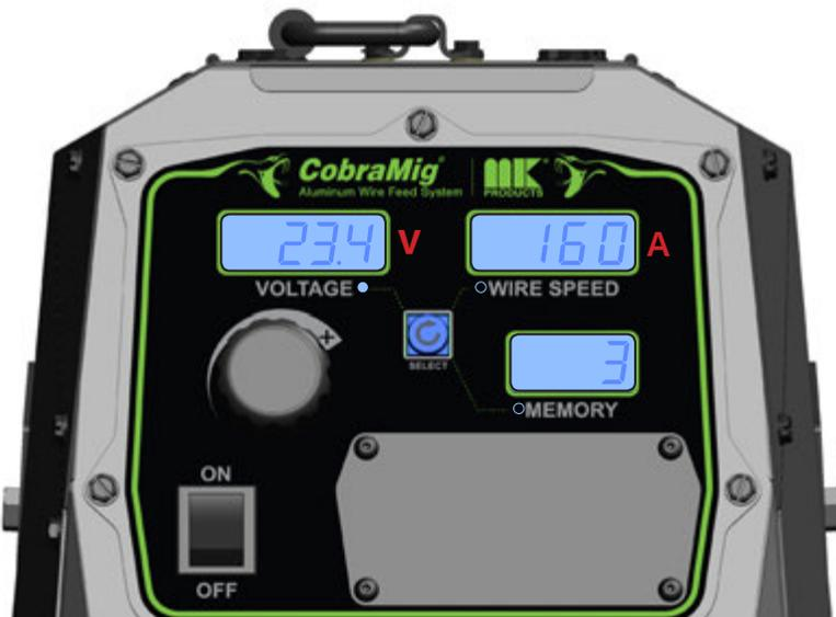
Note: Once arc is established, actual welding Voltage and AMPS will be live and displayed on the user interface for three seconds after weld sequence
