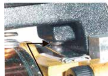
Screw adjusted out of trigger, pre-setting the micro-switch lever for shorter trigger motion sensitivity.
