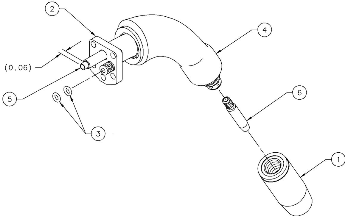
\*Apply silicone lubricant to item 3 before installing.
