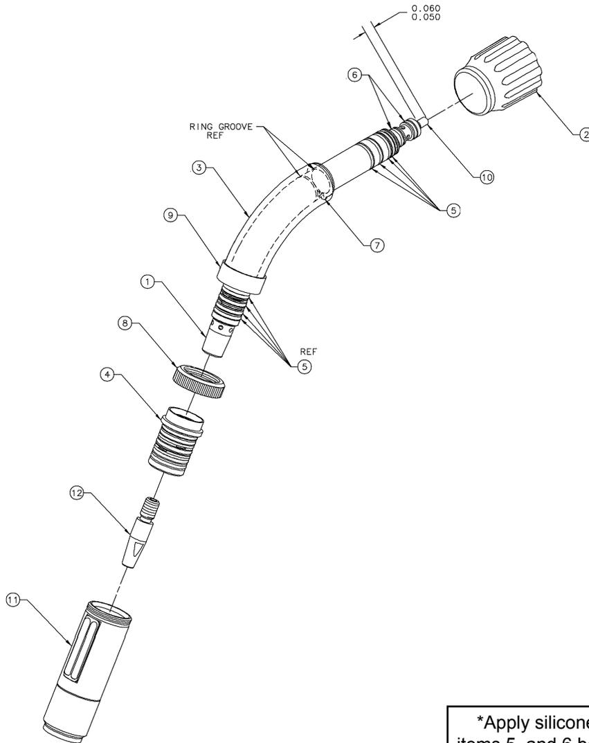
\*Apply silicone lubricant to items 5, and 6 before installing.
