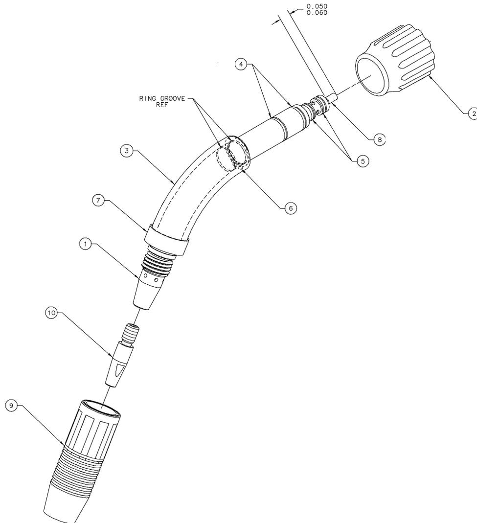
\*Apply silicone lubricant to items 4 and 5 before installing.
