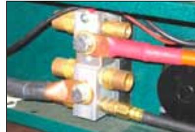
Supplied with this gun is a 3/8-16x5/8" bolt, a 3/8" spring lock washer and a 5/8" flat washer to attach the ring lug to the power block.
