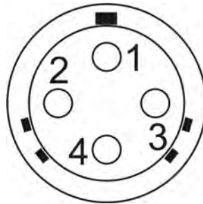
Front Pin View of 4-Pin Circular Connector
